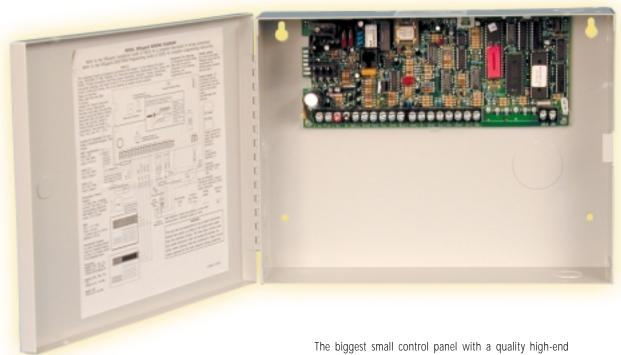
The biggest small control panel with a quality high-end intrusion panel at a low-end price allows you to compete in any market. This remarkable product is expandable to 22 zones, either through wireless or hardwire, has a superior false alarm reduction, and 60-event memory capability. The XRSuper6 is a super panel at a super low price.
